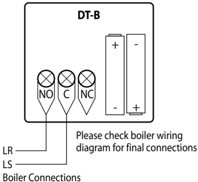
Note: LS & LR may be labelled differently but they are normally the boiler's room thermostat connections.
