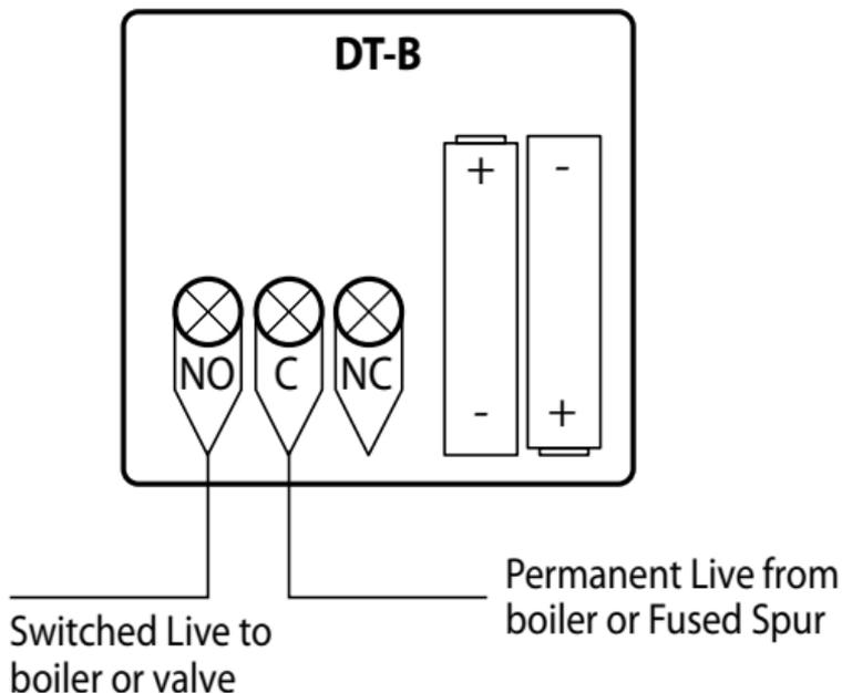
Note: When connecting to a valve, the valve auxiliary switch is used to enable the boiler.
