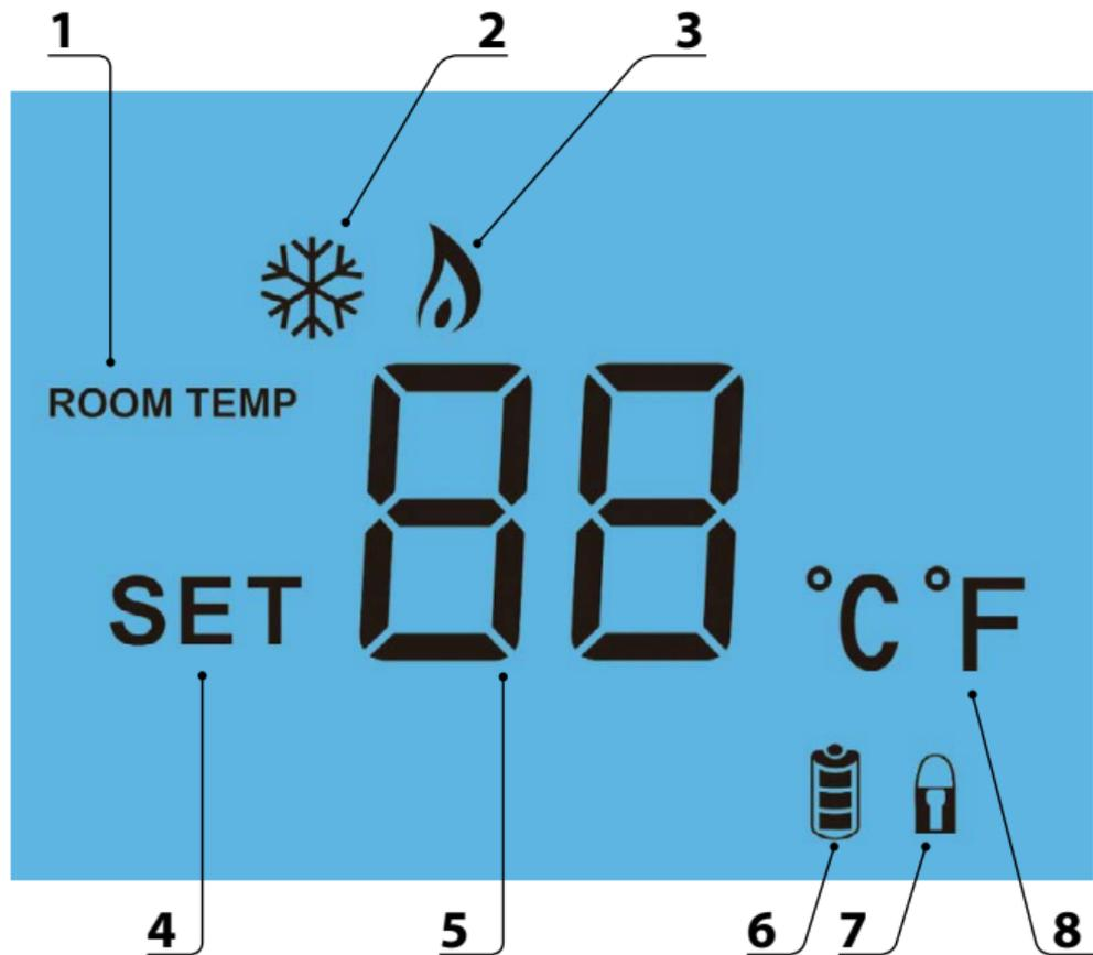
1. Room Temp - Indicates the current temperature sensor mode.
